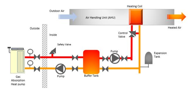
Figure 7: Sample schematic for GAHP heating application with an air handling system
