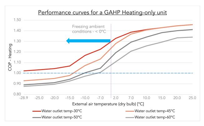
Figure 2: Example of GAHP heating performance relative to ambient air and hot water supply temperatures<sup>14</sup>
