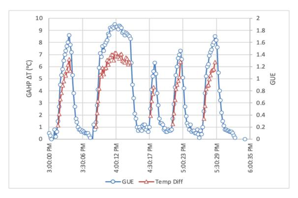
Figure 5: The effect of GAHP differential temperature on GUE
