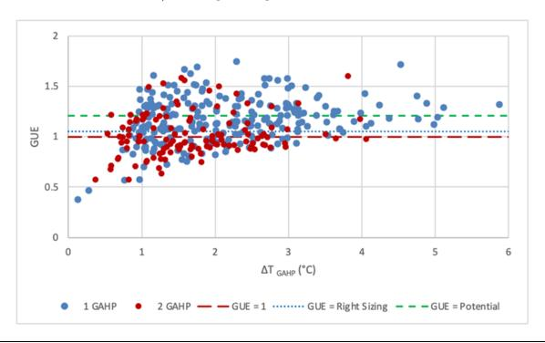
Figure 11: Effect of rightsizing on natural gas utilization efficiency of GAHPs for a DHW system
