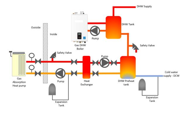
Figure 9: Sample schematic for GAHP application in a DHW system
