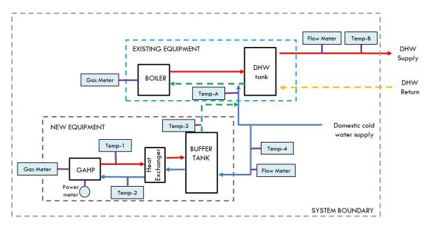
Figure 4: Example of a measurement strategy for savings calculations for GAHPs supporting DHW systems
