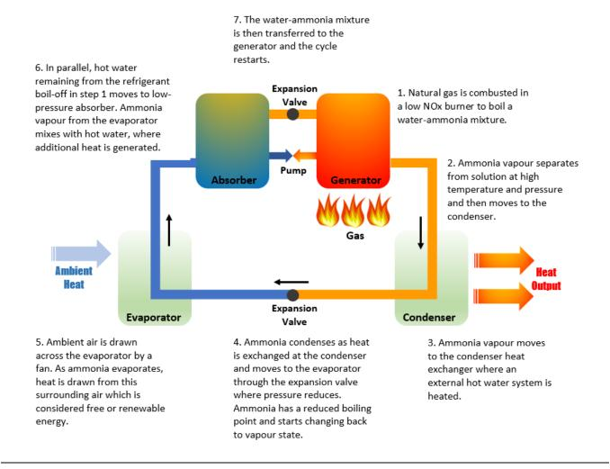
Figure 1: A simplified schematic of the GAHP operating in heating mode
