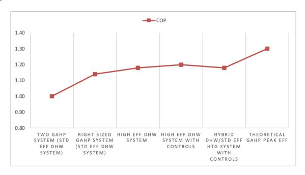
Figure 6: GAHP COPs measured at different phases of the pilot program<sup>31</sup>
