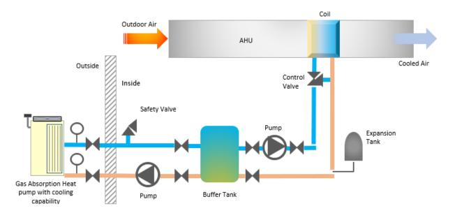
Figure 8: Sample schematic for GAHP cooling application with an air handling system
